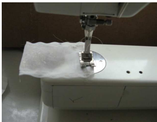
Litterbag construction: Nylon fabric sewed with polyester yarn
