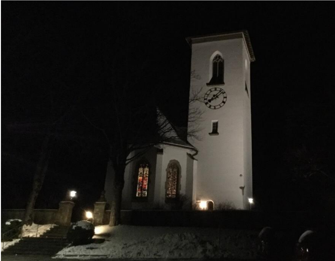
Fig.17 A church with ground-based architectural lighting - much light misses the church or reflects upwards, causing skyglow.
