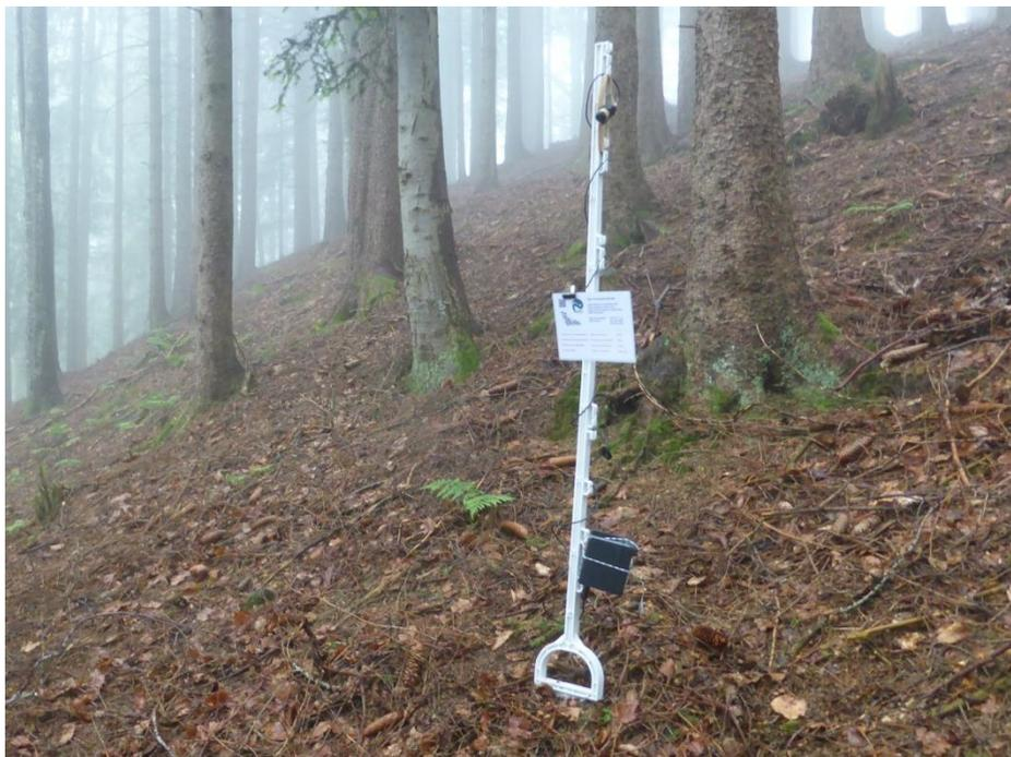
Fig. 4: Batlogger A with information sign and microphone mounted on a pole in Eichberg.
