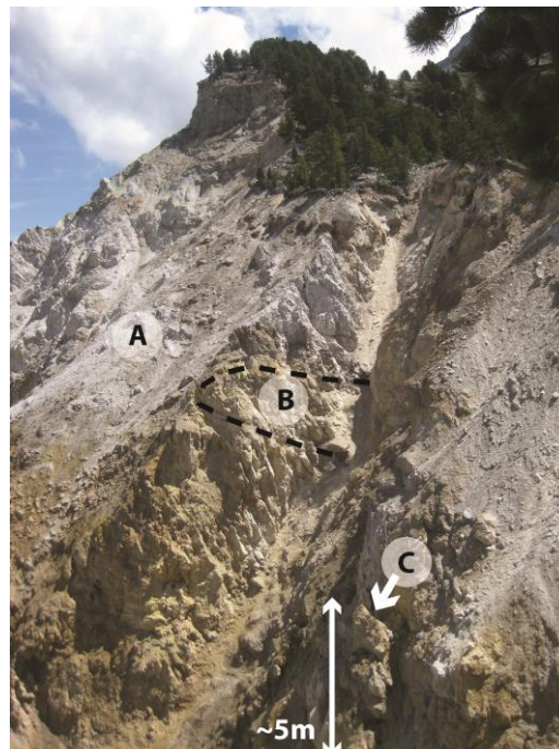
Figure 2.9 – Example of the environment of type (1) failures: the upper 5m of weathered rock and unconsolidated sediment. A = loose sediment cover; B= fold in the quartzites cropping out at the surface; C= imminent failure of ~5m depth.
