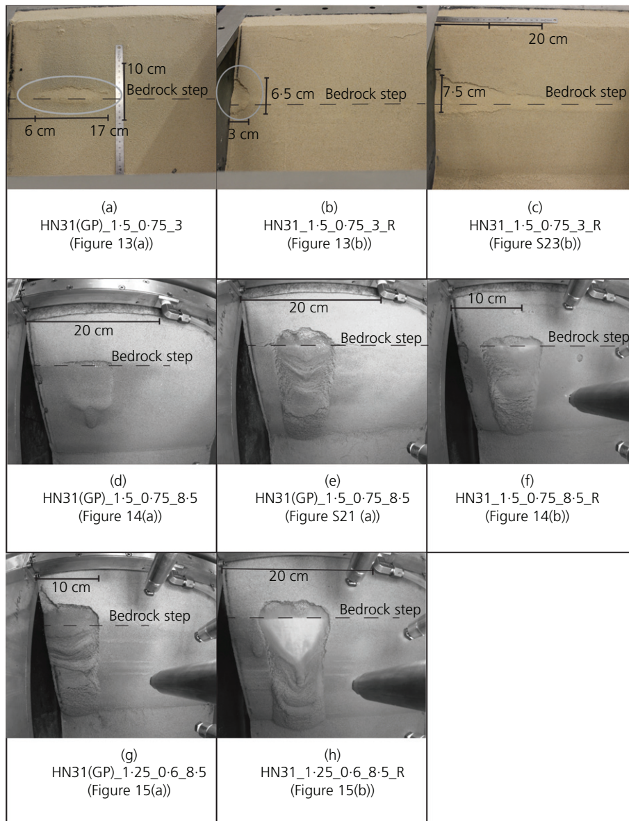
Figure 11. Physical modelling photographs captured after slope failure. (a) Test 2.b, (b) test 3.b, (c), and during failure: test 4.b, (d) test 1.a, (e) test 1.a proof, (f) test 5.a, (g) test 7.a and (h) test 8.a
