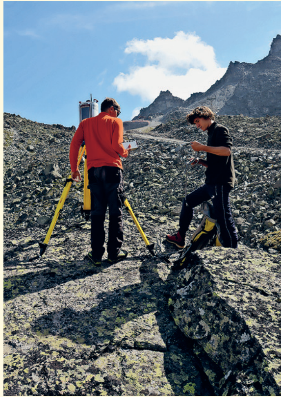
Laser scanning on the Ritigraben rock glacier.
