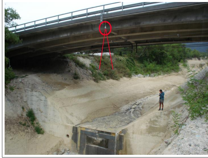
Figure 2.2: Illgraben instrumentation - Force plate and height measuring device
