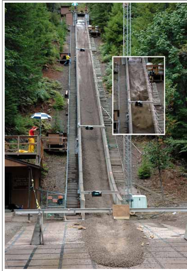
Figure 2.3: U.S. Geological Survey large-scale debris flow flume - the material has just passed the flume mouth and entered the deposition area [59]
