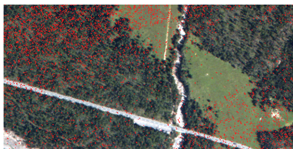
Figure 6: Influence of surface model preprocessing on geometric accuracy: red pixels are shifted in position if a 3x3 smoothing filter is applied to the DSM before geometric processing.
