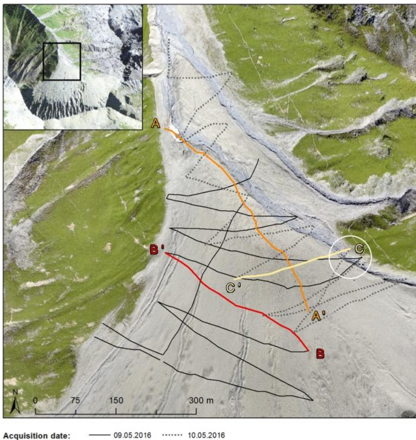
Figure 39: Location of the GPR profiles analysed in this study. Their walking-direction is indicated by the letters (e.g. walking from A to A'). The white circle indicates the ice-rich area from the debris flow 2008.
