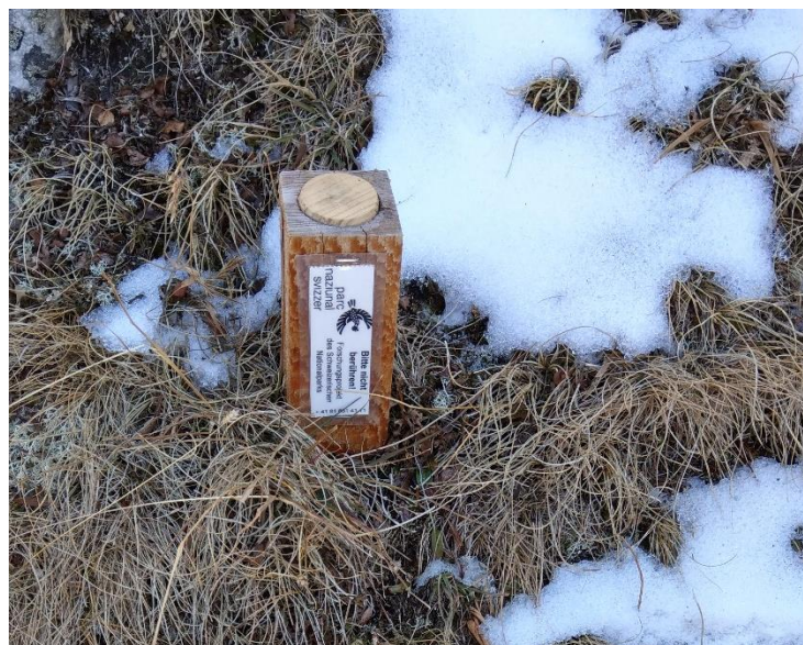
Figure 3 Temperature logger dowel with USB-logger in it
