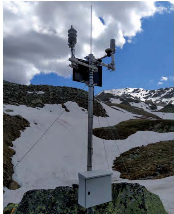
Figure 2 – (Top) The Exosonde, with stainless steel shell and support legs for installation in the lake. The shell and support legs protect the Exosonde from heavy snow/ice and avalanche impact during winter. (Bottom) Instruments set up for recording data from the Exosonde as well as the meteorological station; energy from the solar panel is stored via two batteries in the box. © C. Ebi
