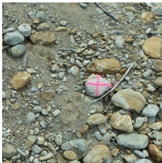
Figure 28. GCP example from the Rio Carlino and clearly visible from the photos, May 2022.
