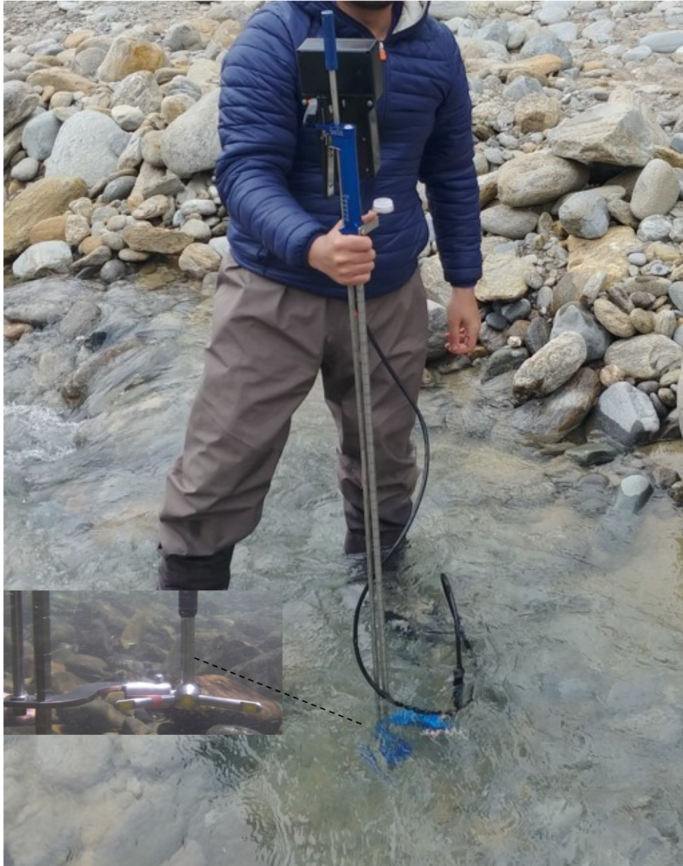
Figure 24. Measuring from Rio Carlino (Flow from right to left) operator stands downstream (facing upstream) of the Flow Tracker, May,2022. Underwater photo from the Flow Tracker manual (flow direction enters the screen)
