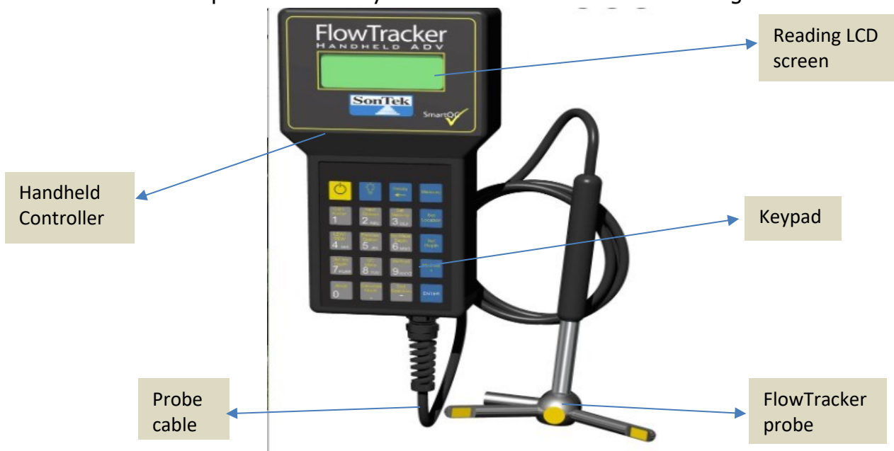
Figure 21. ADV Flow Tracker main components (photo from the Flow Tracker manual)
