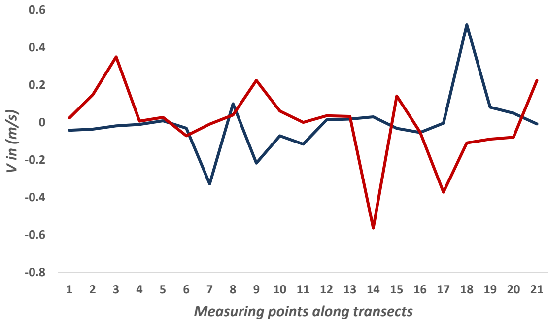
Figure 52. Velocities in the transversal (Y) direction from two rapid units from Rio Carlino. The red graph represents the data from rapid nr.2 and the blue the data from rapid nr.3
