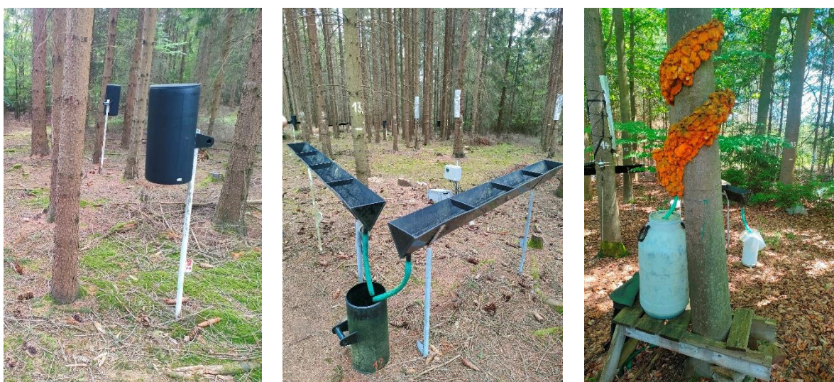
Figure 6-1: Snow samplers (left) and throughfall sampling gutter system (center) in a Level II plot with Norway spruce and stemflow sampler (right) in a European beech plot near Žďár nad Sázavou, Czechia. Images: Arne Verstraeten
