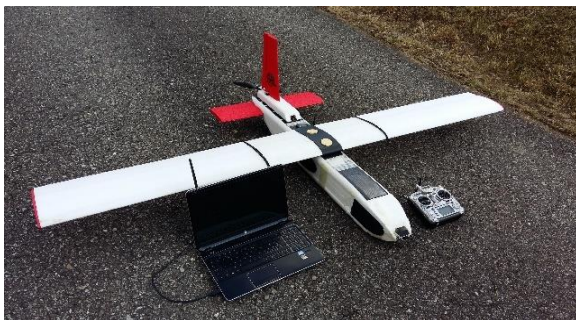
Figure 1 - Our Maja D fixed-wing drone from Bormatec with a laptop containing a telemetry link as ground station and the remote control. © S. Weber 2016
