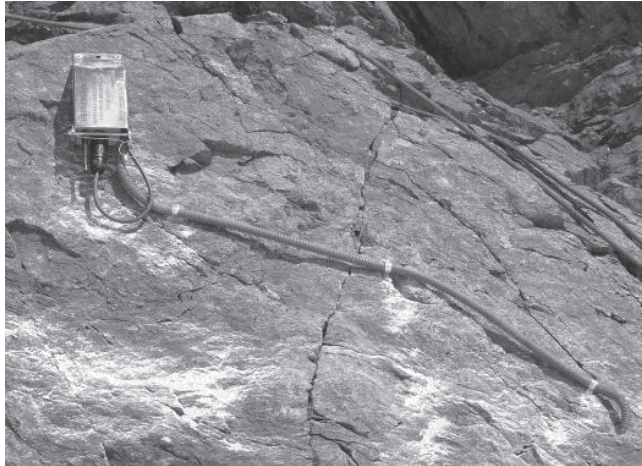
Figure 5. Network node #4 and cable to the sensor rod, which is drilled one meter into the rock perpendicular to the surface. The network nodes can be easily exchanged and attached to the sensor by a waterproof plug.
