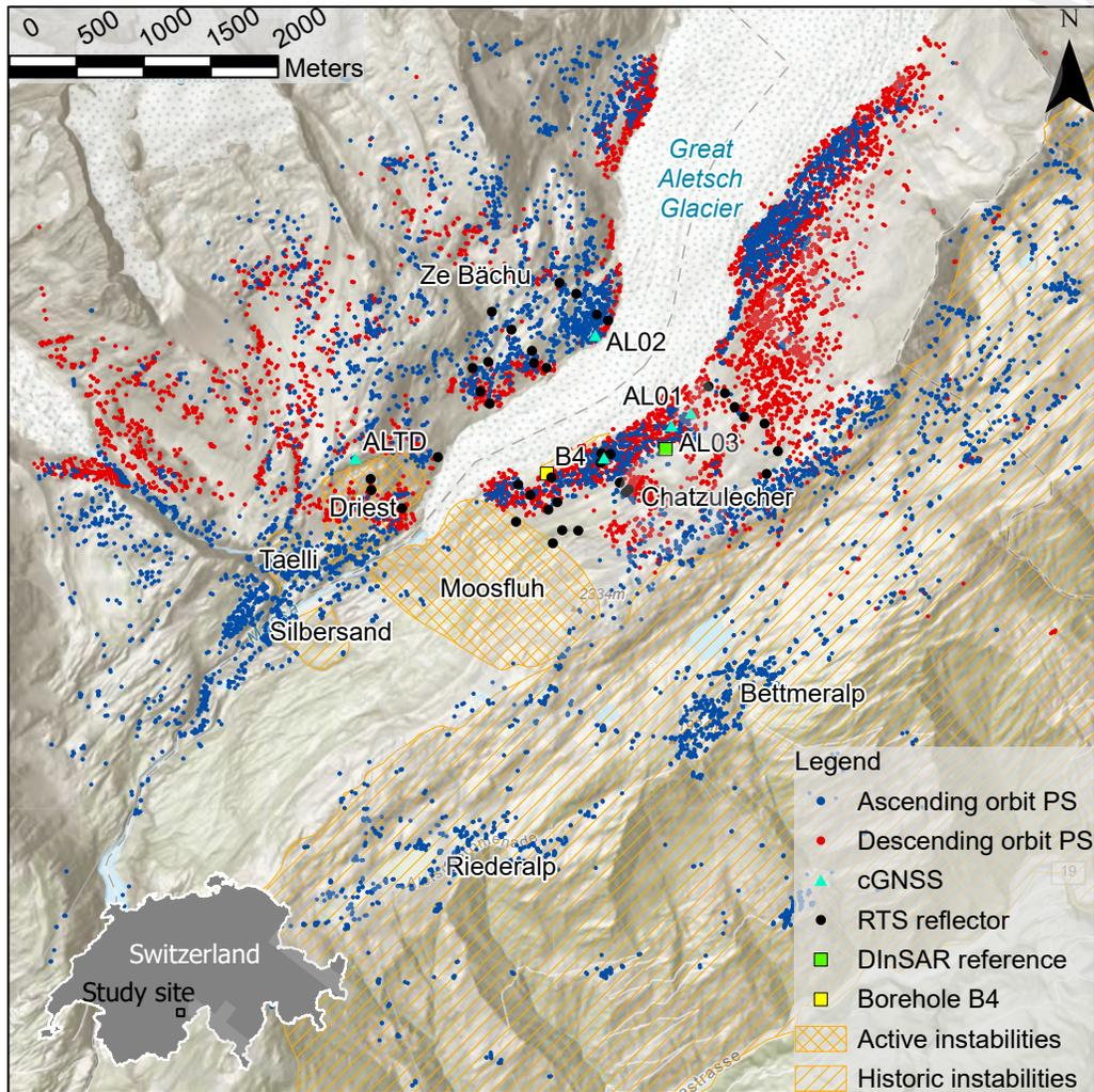
Figure 1: Study area with selected Persistent Scatterers (PS) for the analysis of the ascending (blue) and descending (red) orbits and the DInSAR reference point (green rectangle). cGNSS stations (cyan triangles), RTS reflectors (black points), and the borehole (yellow square) used in this study are drawn around the tongue of the Great Aletsch glacier, close to a range of large instabilities (orange patches). The location of the study area in Switzerland is shown in the bottom left corner.
