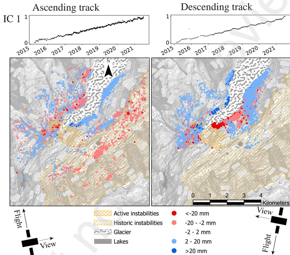
Figure 3: First independent component of vbICA for the ascending and descending tracks of the satellite. The upper panels show the time series of the IC. Positive values (blue colored dots) on the map signify displacement towards the satellite for a positive change in the time series. To reconstruct the displacement associated with the IC at a PS between two dates, multiply the value shown on the map by the difference in the time series of IC1 (upper panels) at the two given dates.
