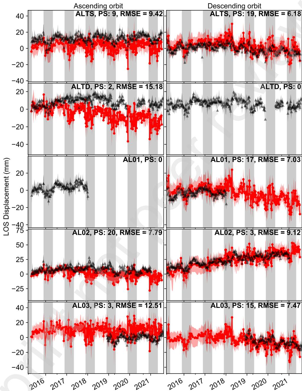
Figure 2: Comparison between cGNSS stations displacement (black) and nearby permanent scatterers (red) for the ascending (left) and descending (right) orbits in a circle of 50 m radius around each station. See Figure 1 for the location of the five cGNSS stations. PS is the number of permanent scatterers in the 50 m circle around cGNSS stations, RMSE is in mm. Grey zones mark times when the stations are susceptible to being snow-covered, inducing a larger scattering of the satellite recordings.
