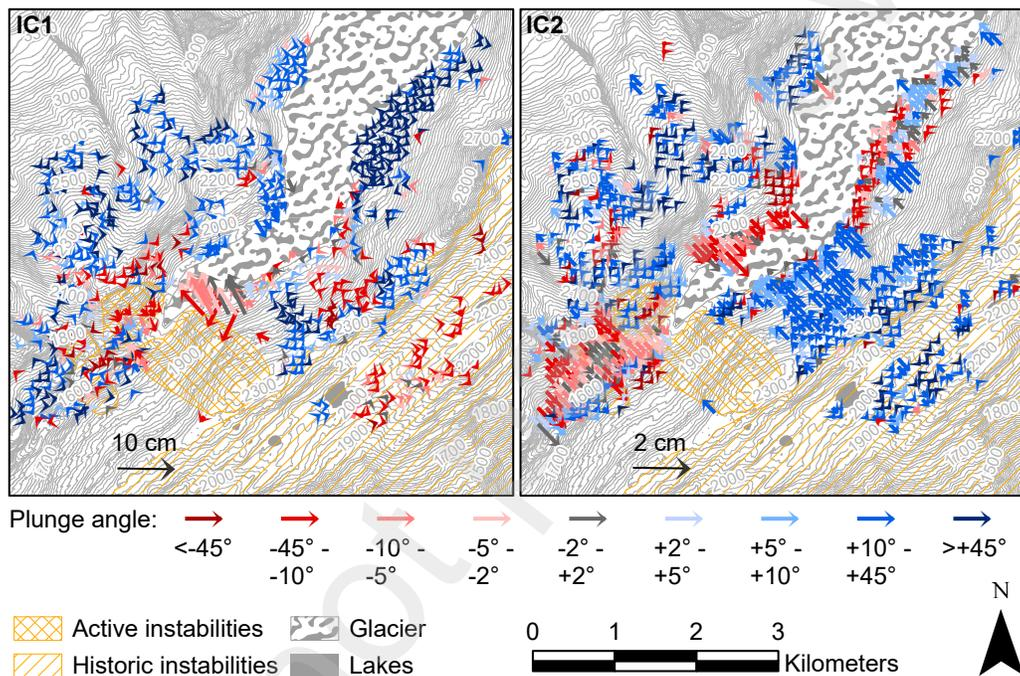
Figure 7: Displacement obtained by combining the ascending and descending orbits with the local average slope direction for the first IC (left) and with the average dip direction of the foliation for the second IC (right) of the vbICA method. The arrows show the horizontal orientation of displacement and magnitude (long-term trend for IC1, during recharge for IC2), and the colors display the plunge angle of the displacement.
