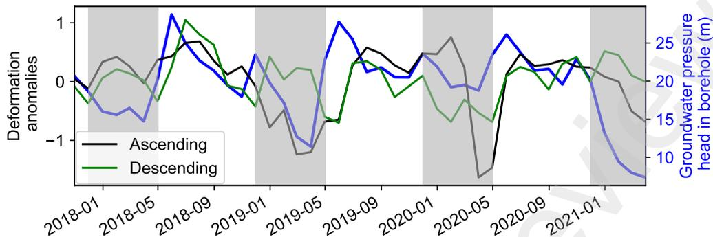
Figure 5: Comparison between the monthly deformation anomalies (ascending orbit, black and descending orbit, green) and the monthly pressure head at B4 (blue). Grey areas are periods with expected partial snow coverage, during which lower correlation factors may be expected because of decorrelation induced by the snow.
