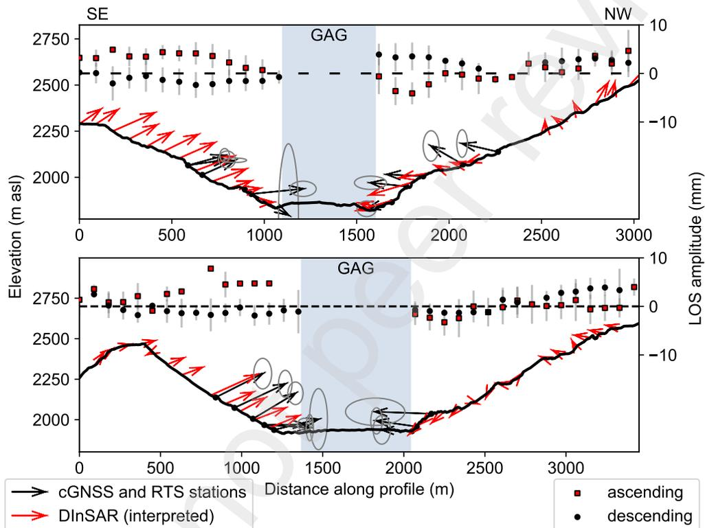
Figure 6: Topographic profiles across the valley with groundwater-related displacement during infiltration. Top: profile 1; Bottom: profile 2 in Figure 4. Black arrows are cGNSS and RTS data (grey ellipses for uncertainty). Red arrows are interpreted direction of ground displacement from DInSAR, and points are raw data from Figure 4 with a 90 m buffer distance around the profile. GAG stands for Great Aletsch Glacier, and its extent is delimited in blue.
