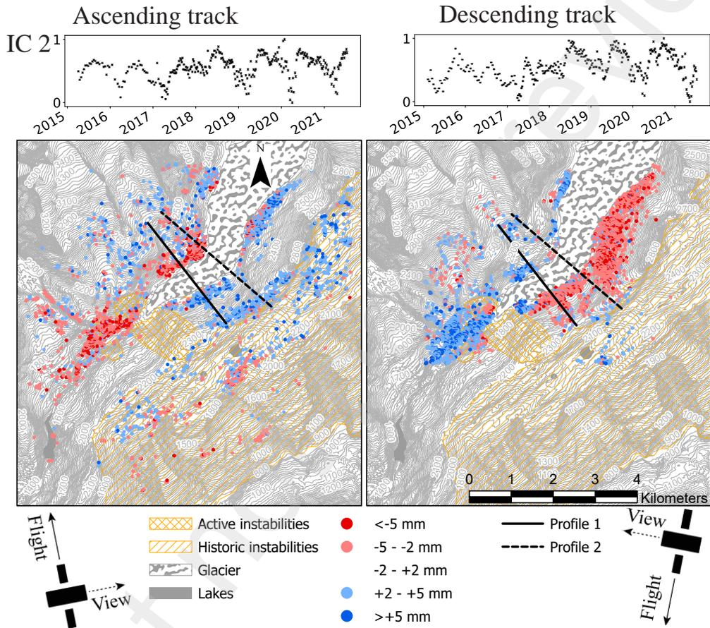
Figure 4: Second independent component of vbICA exhibits cyclic annual displacement for the ascending and descending tracks of the satellite. The upper panels show the time series related to the IC. Positive values on the map signify displacement towards the satellite for a positive change in the time series.
