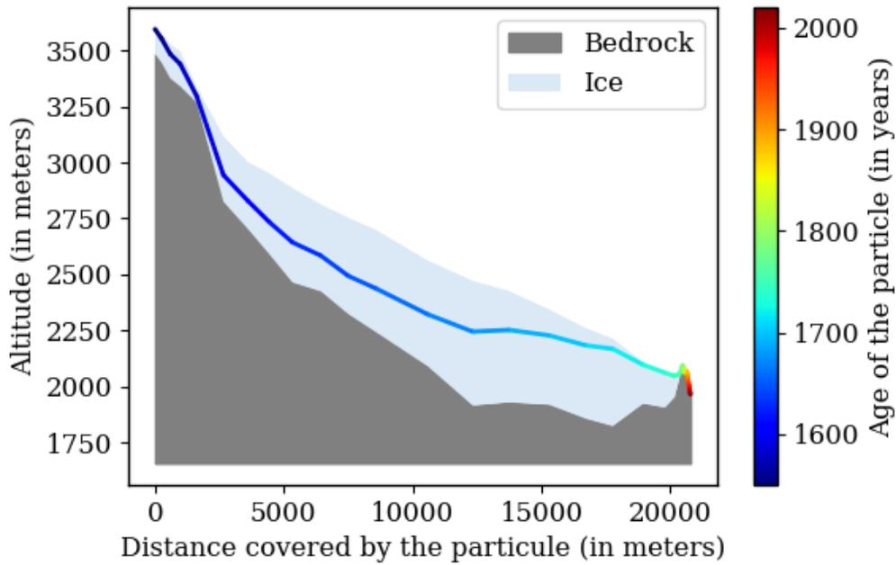
Figure 20: Trajectory of a particle in Aletsch glacier with kinematic method
