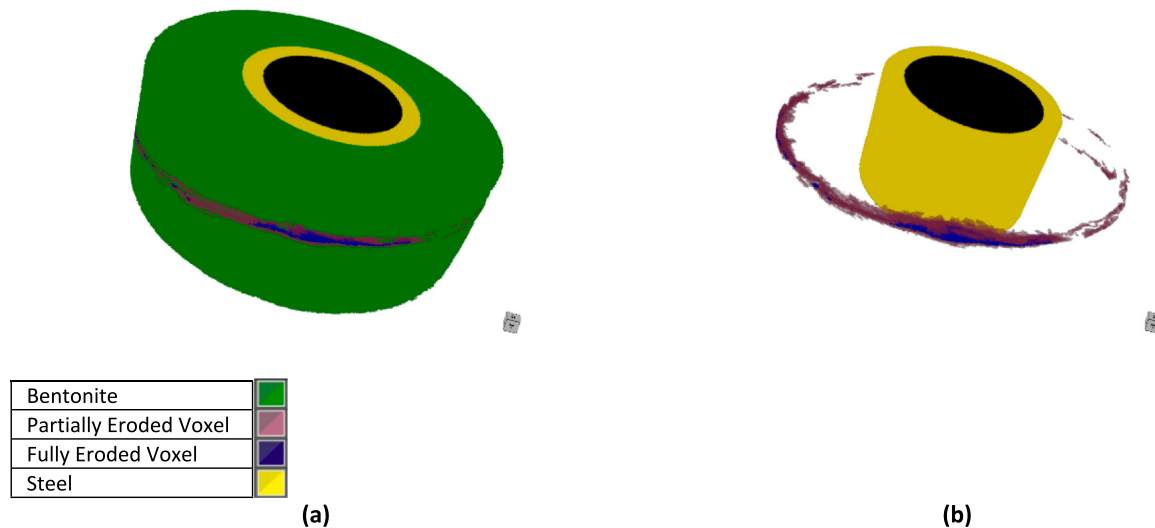
Fig. 9. a) 3D segmentation results using the RF algorithm for erosion evaluation. A cylindrical mask was applied around the FEBEX rings. b) The same as (a) but the bentonite voxels were not shown for comparison purpose.
