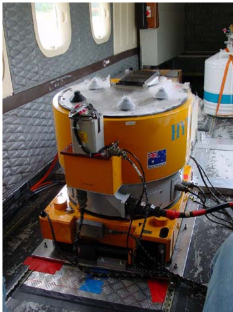
Fig. 2: HyMap in its stabilised platform mounted in a DLR Do-228
