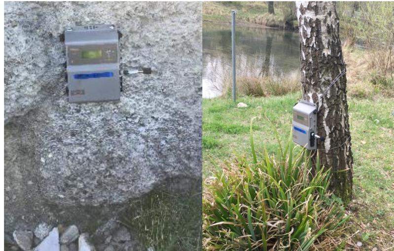
**Figure 3:** Left: recorder mounted on a wall in the enclosure in Männedorf. Right: recorder on a tree in Tierpark Dählhölzli.
