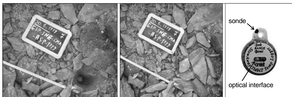
Fig. 8.12 Temperature data loggers: Mini data loggers for T are buried in the substrate at -10 cm. Left, logger position opened. Centre: logger position closed. Right, StowAway Tidbit temperature logger (compare Fig. 8.10).
