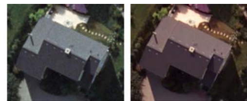
Figure 70: left: image from analog camera, right: same area mapped with UltracamD (from Perko, 2006)
