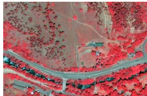
Figure 16: Color Infrared satellite image (0,6 m / 2,4 m ground resolution; www.digitalglobe.com )
