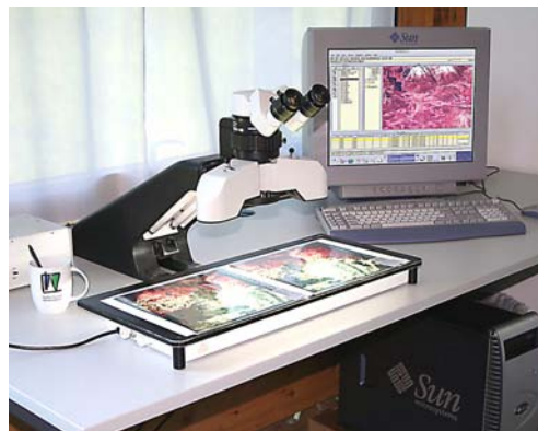
Figure 12: Professional GIS workstation with a high quality stereoscope (Wild APT1, LIZ)
