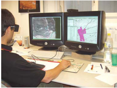
Figure 18: Digital photogrammetry workstation: on the left screen the stereo image display can be viewed by the aid of special eyeglasses, on the right screen appears the mapping in the GIS. (Hauenstein/Jörimann)
