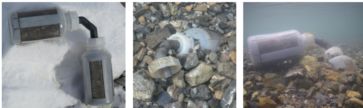
Figure D.2.10: Combined incubation-emergence box-traps to investigate the success of emerging larvae
