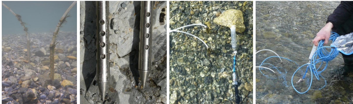
Figure D.2.7: DO steel pipes with perforating tops and PVC-tubes used to suck interstitial water and measure the dissolved oxygen concentration in two sediment depths (10 cm, 20 cm)
